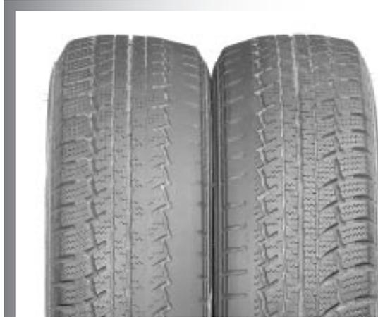
*Increased, one-sided wear due to "slip". It is frequently encountered in connection with a worn tread surface. This is also often seen together with burrs along block edges up to worn tyre shoulders.*
