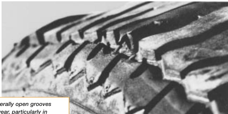
Tyres with large blocks or laterally open grooves are susceptible to stepped wear, particularly in non-powered wheel positions. The blocks exhibit more pronounced wear on the rear edge (relative to the direction of tyre rotation) than on the front (leading) edge, giving the blocks a characteristic saw-tooth wear pattern when viewed from the side.
