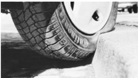
**Tip** Kerbs and similar obstacles should only be driven over at an obtuse angle and at appropriately slow speed.
