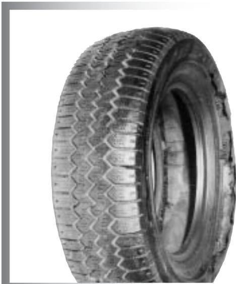
*Major heat build-up in the tyre due to driving in an underinflated state led to separation of structural components and to melt-down of the rubber.*
