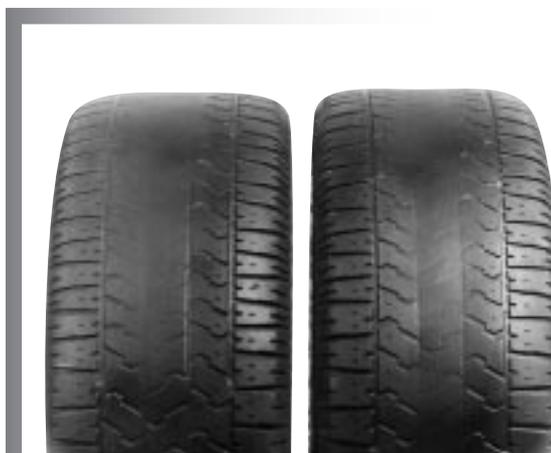
*Example of tyre wear pattern on powered axle of a powerful car: pronounced wear is visible in the tread centre.*
